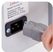
IEC power cable into the mains.
