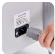
IEC power cable into the mains.
