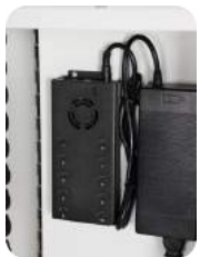
Isolated power compartment for electrical safety
